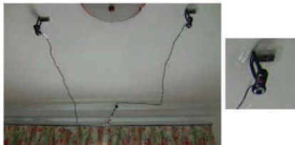
(b) Ceiling cameras for the vision-based tracking system.
